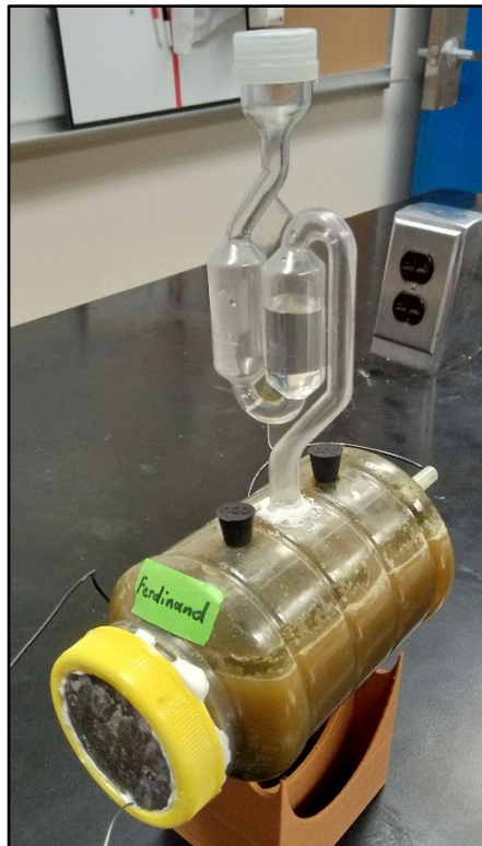
Figure 3. Isometric View Photograph of Microbial Electrolysis Cell
