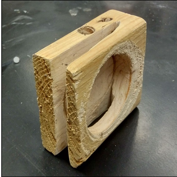
Figure 15. Completed Geiger Tube- and Shield-Holder Apparatus
