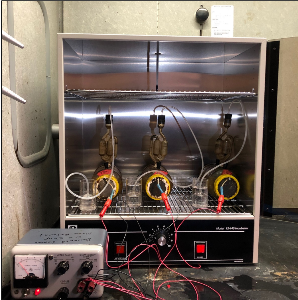
Figure 17. Microbial Electrolysis Cells Generating Hydrogen in Incubator
